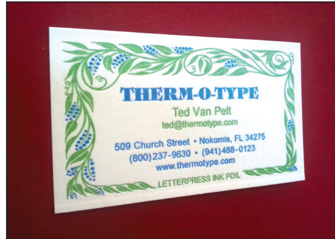
Letterpress ink Foil applied on a business card using the NSF Elite Foil Press.
