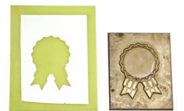
Counter cast masking vinyl can dramatically reduce the time required to produce a cast counter.
