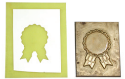
Counter cast masking vinyl can dramatically reduce the time required to produce a cast counter.
